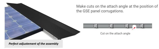
3 Place the top junction flashing, having applied beforehand two PU glue joints on the covered top flashing area. The connecting piece must overlap with the top flashing with at least 100 mm. The gap between the top flashings should not exceed 160 mm.
