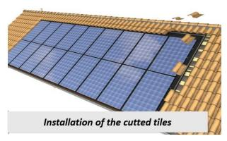
It may be necessary to cut the tiles to ensure a compliant overlap between the elements, according to roofing regulation. These elements must be attached mechanically, as described in the roofing regulation.
