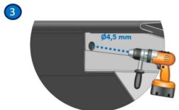
Once the height adjusted, drill the overlapped pieces with a 4,5mm drill bit
