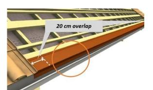
The connection of the waterproofing strip to the gutter can be done with a drip flashing: one for the PV field, another one for the roof underlayment.
