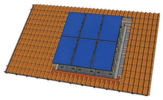
1 Position the modules in such a way that they are resting on the support pads and abut against the upper pads (orange arrows).
