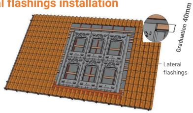
WARNING: BEFORE INSTALLING THE LATERAL FLASHINGS, MAKE SURE TO PLACE THE WEDGES AT THE ARRAY ENDS, UNDER THE CORRUGATIONS, WHERE THE END CLAMPS ARE LOCATED.
