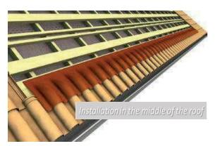
A batten is placed to fit with the thickness of the roof tile and to provide a flat base for the sealing strip.
