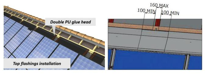
4 In the same way, place the corner flashings, having applied beforehand a PU glue joint on the overlapping zone of the top flashing. (Overlapping at least 100mm)
