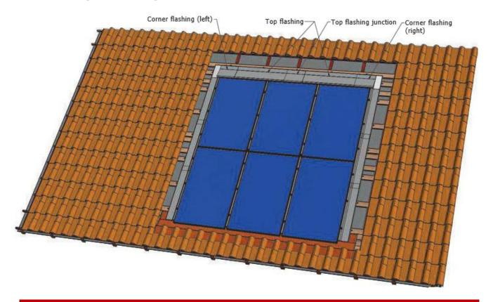
WARNING: THE TOP FLASHING PIECE IS DESIGNED WITH A SLOPE OF 14° TO ALLOW WATER FLOW ABOVE THE UPPER ROW OF MODULES. IT IS THEREFORE, ESSENTIAL FOR THE INSTALLER TO ENSURE THAT THE ROOF SLOPE IS SUFFICIENT TO PREVENT WATER RETENTION ACCORDING TO THE REGULATION.
