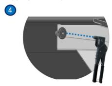
Assemble the pieces with a rivet
