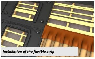
Then, position the GSE panel so that it's overlapping with the flashing strip.
