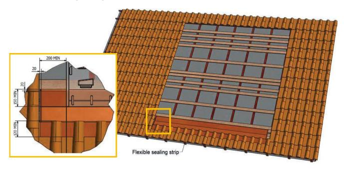
The sealing strip is laid out to link up with the bottom part of the roofing (PV array in the middle of the roofing).
