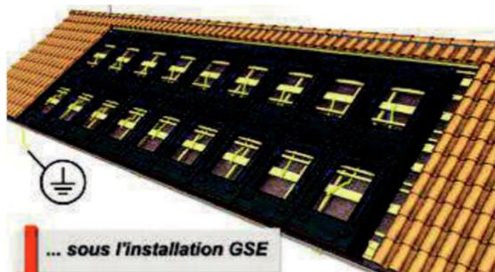
**ATTENTION : LORS DE LA MISE EN PLACE DES CABLES, VEILLER A NE CREER AUCUNE BOUCLE D'INDUCTION, CONFORMEMENT AUX GUIDES UTE C15-712**
