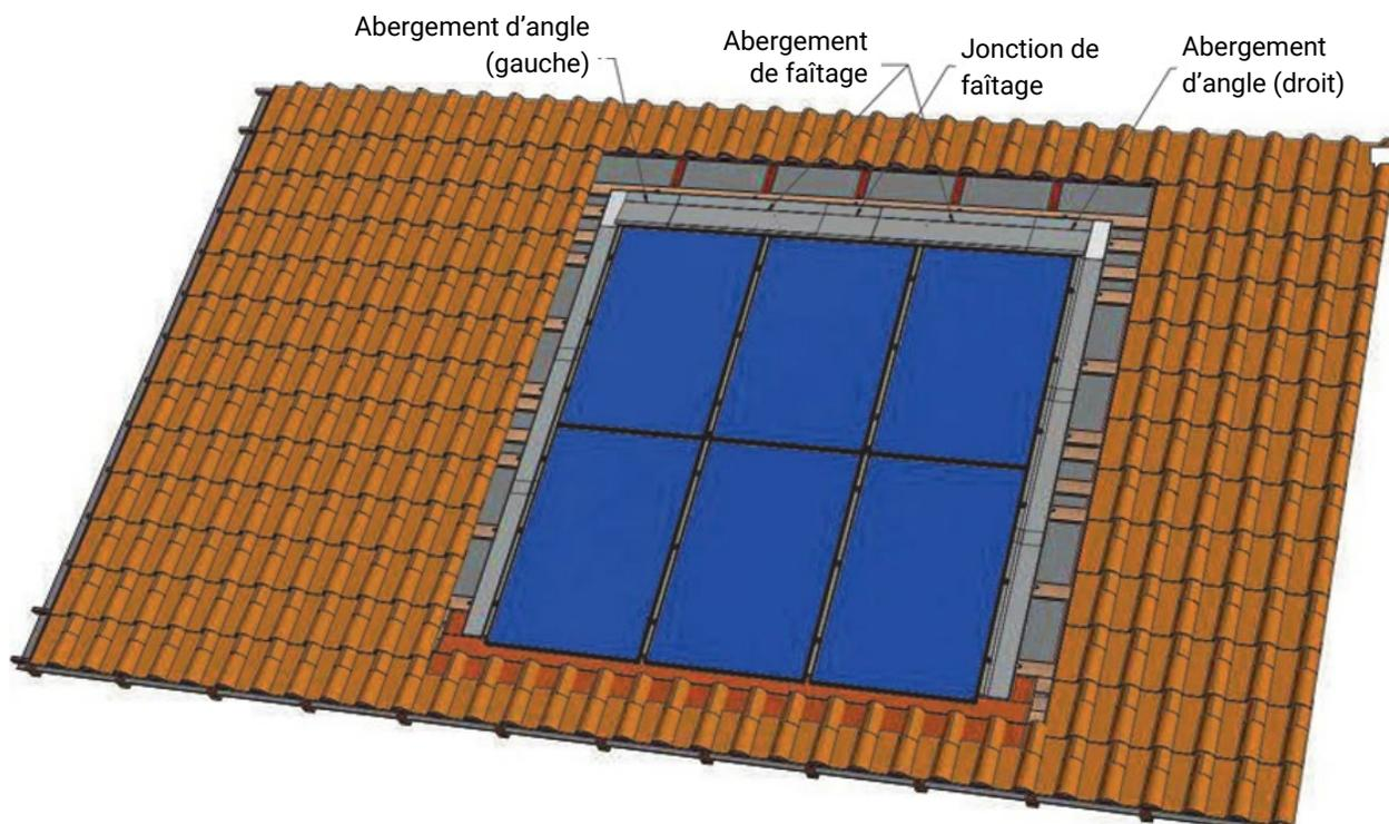
**ATTENTION:** LA PIÈCE D'ABERGEMENT DE FAÎTAGE EST CONÇUE AVEC UNE PENTE DE 14° QUI PERMET DE FACILITER L'ÉCOULEMENT DES EAUX AU-DESSUS DE LA DERNIÈRE RANGÉE DE MODULES. IL EST DONC PRIMORDIAL QUE L'INSTALLATEUR S'ASSURE QUE LA PENTE DE TOITURE SOIT SUFFISANTE POUR NE PAS CRÉER DE ZONE DE STAGNATION DE L'EAU CONFORMEMENT AUX DTU COUVERTURE.
