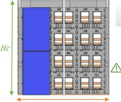
$Hc\ (mm) = (Height\ Ref. + Intermodule\ Graduation) \times nb.rows + 310$  $Lc\ (mm) = (Width\ Ref. + 40) \times nb.columns + 310$
