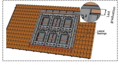
Straight to the clamps position, pre-drill through the flashing, plastic frame and wedge.
