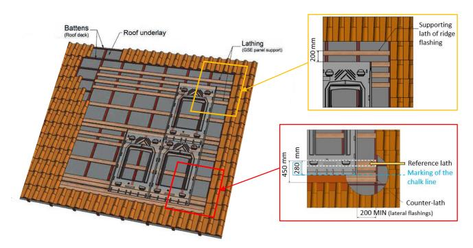
The sections of the support battens are determined according to climatic loads.
